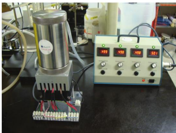
Figure 7 First Generation Stainless Steel DUV LED Water Disinfection Chamber. Adapted from IUVA 2012“Integration of Deep Ultraviolet Light Emitting Diode Technology into Point-of-Use Drinking Water
